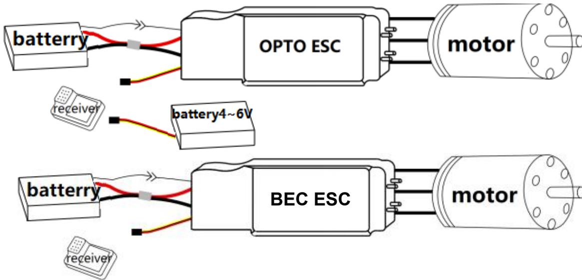
① The above drawing show how to connect the ESC with all the other parts.
